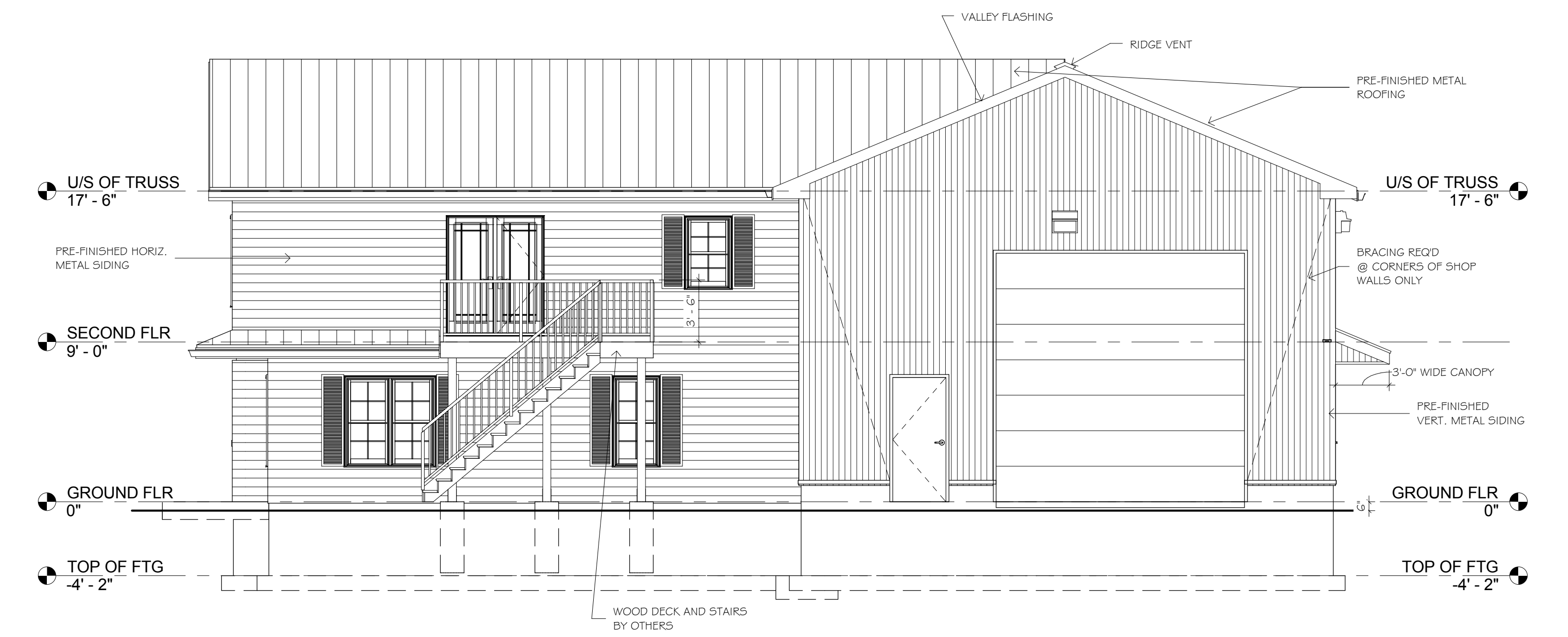
- SOUTH ELEVATION A1/A3 / 3/16" = 1'-0"
